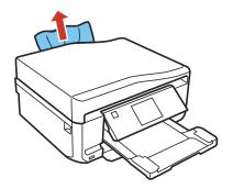
3. Lift the scanner unit and remove any jammed paper inside.
